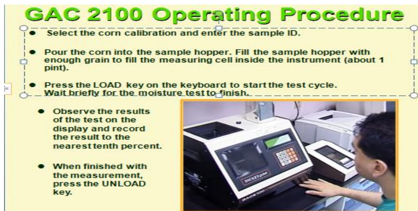
Fig. (1): GAC 2100 device for moisture content determination.
